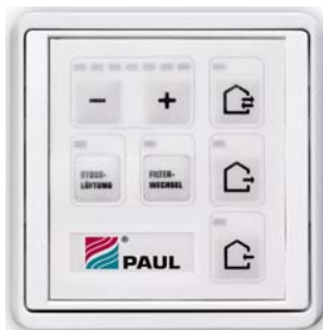
Version 2: Plastic film keyboard for manual operation (LxWxD in mm: 80x80x12); Cable: IYSTY 2x2x0, 6, max. 15 m, provided by customer
