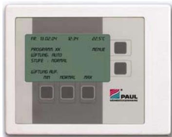
Version 1: Comfort operating element for automatic operation (LxWxD in mm: 158x125x32); at the low point Cable: IYSTY 2x2x0, 6, max. 15 m, provided by customer
